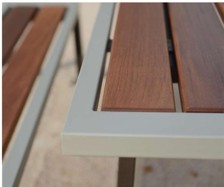
80 x 40 mm and 40x40 mm steel tube frame. Wooden elements with 120 x 35 mm section. Sealed at 4 points. Compliant with standard NF P99-610, category "S".
