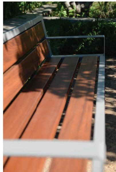
80 x 40 mm and 40x40 mm steel tube frame. Wooden elements with 120 x 35 mm section. Sealed at 4 points. Compliant with standard NF P99-610, category "S".
