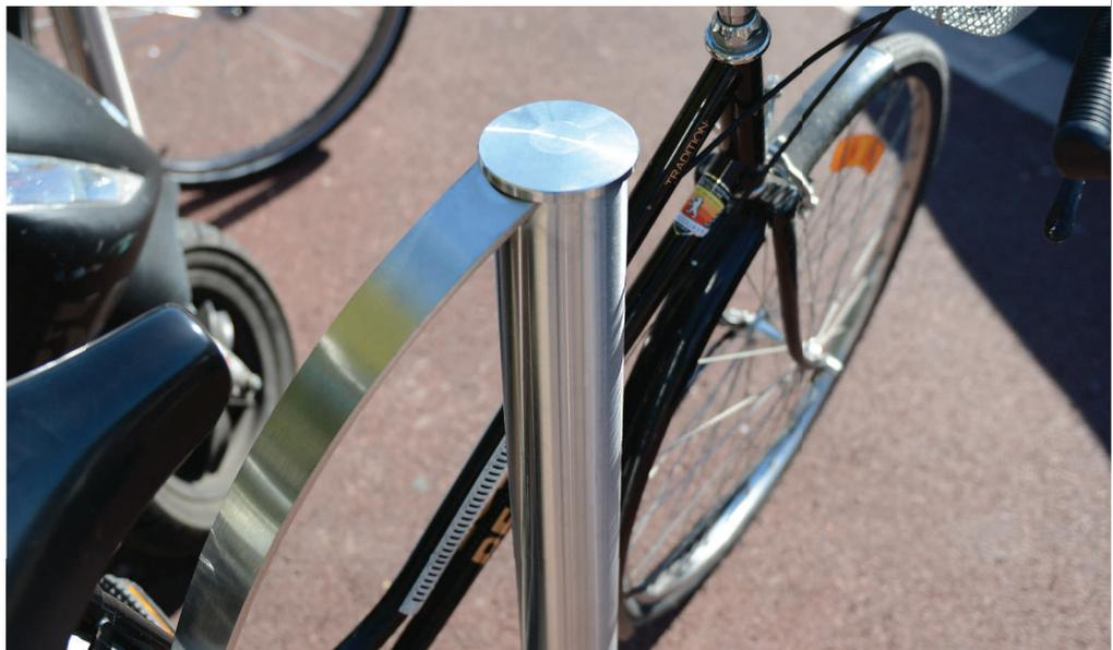
Model made from stainless steel tube  $\varnothing 76$  mm. Machined solid stainless steel head  $\varnothing 86$  mm. Flat curved 50 x 6 mm. Depth of seal 200 mm.
