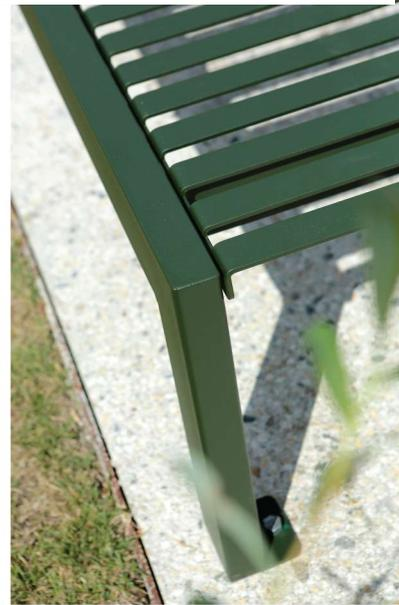
Steel tube leg frame, 80 x 40 mm. Sheet steel seat and back rest, 5 mm thick, welded to leg frame.
