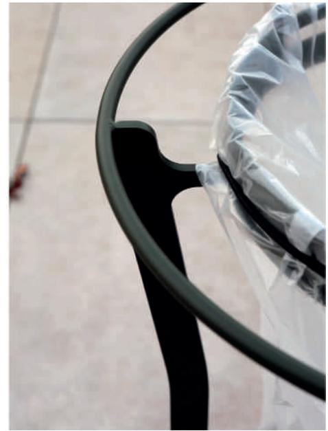
Bin with support system for 100 litre bag. Made from flat steel profiles, 5 mm thick and steel sheet, 2 mm thick.
