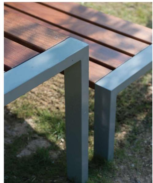
Steel tube leg frame, 80 x 40 mm. Wooden elements with 120 x 35 mm section. Sealed at 4 points. Compliant with standard NF P99-610, category "S".
