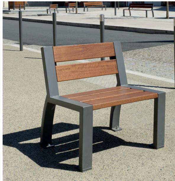
Steel tube leg frame, 80 x 40 mm. Wooden elements with 120 x 35 mm section. Sealed at 4 points.
