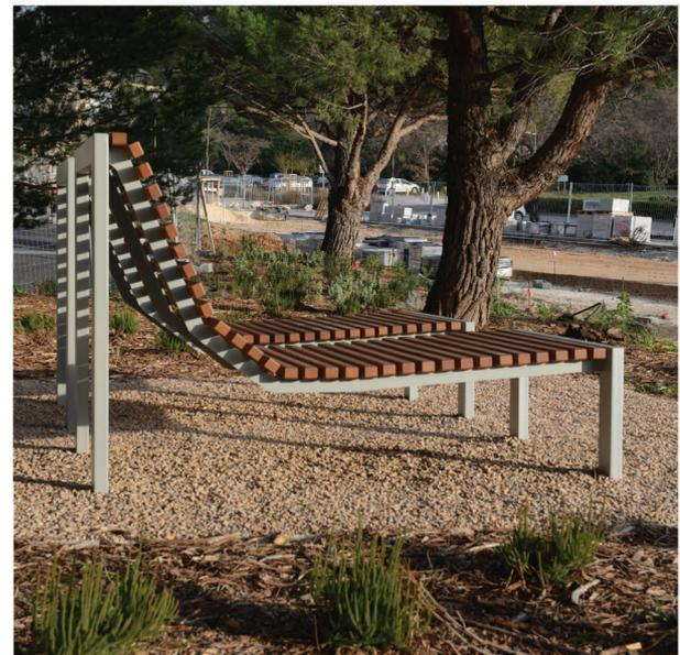
Steel tube leg frame, 80 x 40 mm. Wooden seat and backrest, 38 x 35 mm section. Sealed at 4 points. Compliant with standard NF P99-610, category "S".
