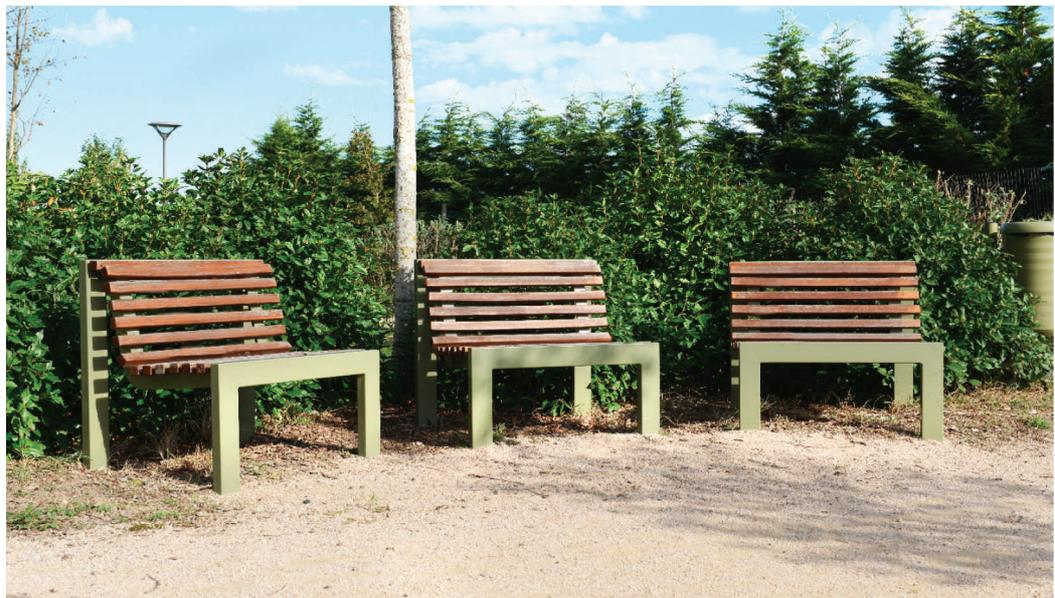
Steel tube leg frame, 80 x 40 mm. Wooden seat and backrest, 38 x 35 mm section. Sealed at 4 points. Compliant with standard NF P99-610, category "S".
