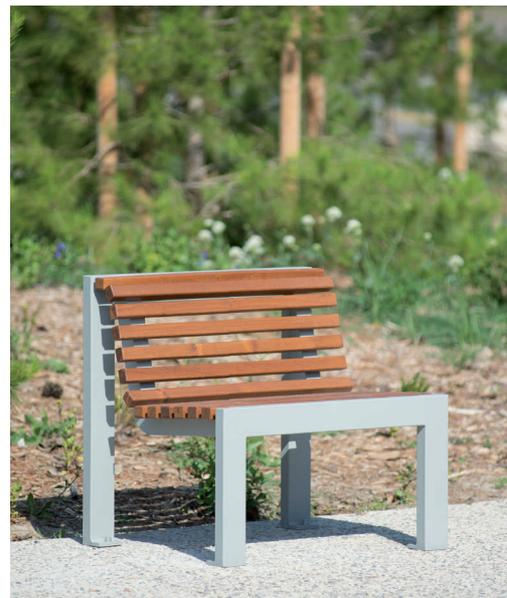
Steel tube leg frame, 80 x 40 mm. Wooden seat and backrest, 38 x 35 mm section. Sealed at 4 points. Compliant with standard NF P99-610, category "S".
